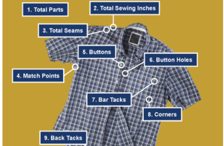
Information on common construction details is used to calculate manufacturing time and labour cost
